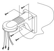
2. Pull the safety cable that is fixed to the housing outside of the housing.
