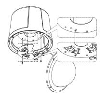
Connect the safety cable from the housing to the internal fixture ring of the STH-270PWV wall mount.
