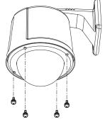
11. Make sure that all the devices are connected correctly to the camera and then check the functions of the camera. If there are no problems, affix the housing onto the wall mount using the three screws.
