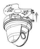
9. Assemble the speed dome by turning it in the direction of the arrow.
