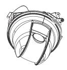
10. Install the dome cover for the speed dome's outdoor housing.
