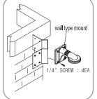
3. Fix the wall type mount(STB-270PWV) with four 1/4 inch screws.
