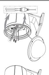
7. Connect the video cable, the controller cable, the camera power adapter cable and the ID setting cable to the speed dome camera.
