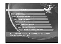
You can select the satellite and LNB setting conditions to execute channel search and you can alter the settings for 22KHz tone. The parameters set in this menu are needed for programming the channels for the "**Auto scanning**" and "**Manual scanning**".
