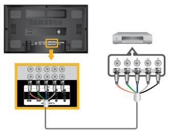
1. Connect the [BNC/COMPONENT IN [R/Y, G/P<sub>B</sub>, B/P<sub>R</sub>]] ports on the monitor to the BNC port on the external device using the BNC to BNC cable.
