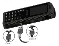
Note: The previous illustration is the correct and incorrect method for connecting the charger. If the incorrect method is attempted, damage to the accessory port will occur therefore voiding the phone's warranty.
