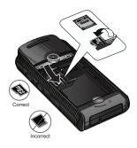
**Warning!:** Please note the printed circuit side faces down when inserting the card.
