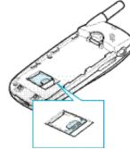
6. Place the battery back on the phone. Slide the battery up towards the catch until it locks into place. Make sure that the battery is properly installed before switching on the power.
