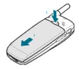
3. Slide the ivory-coloured lock on the SIM card holder left to unlock the holder. Lift the holder up.
