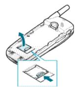
Insert the SIM card, ensuring that the cut corner faces top left and the gold contacts of the card face into the phone
