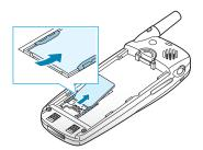
4. Place the battery back on the phone. Slide the battery up towards the catch until it locks into place. Make sure that the battery is properly installed before switching on the power.
