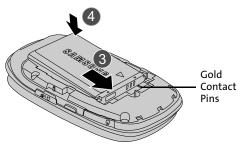
4. Gently press down on the battery until it snaps into place (4).
