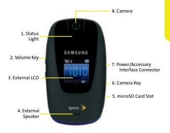
Status Light illuminates while the battery is charging, and blinks when a new message or phone call is received.
