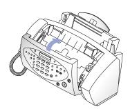
**Replace the roller in reverse order**, and then close the Control Panel firmly until it clicks into place.
