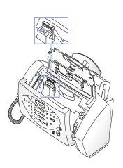
**Re-install the Cartridge** and close the Cover and Panel.
