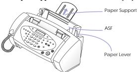
Before loading papers, **push down the blue Paper Lever.**Failure to do so will result in paper jams while copying or receiving a fax.
