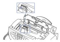
Close the cover and replace the Control Panel after installing the print cartridge.
