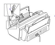
**Disassemble the White Roller**. At the right-hand end of the White Roller there is a bushing that is secured with a small white tab. Push the tab slightly inward, then rotate towards you. Then pull up the right-hand part to take it out.
