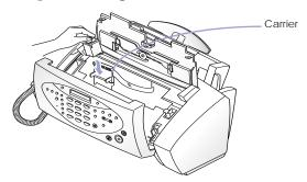
**Push the cartridge firmly** in the direction of the arrow until it clicks into place.
