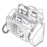
Clean the Cartridge Carrier contacts and Deflector (metal piece) with clean and dry cloth.
