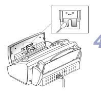
**Clean the ADF Rubber piece** at the back of the Control Panel, too.
