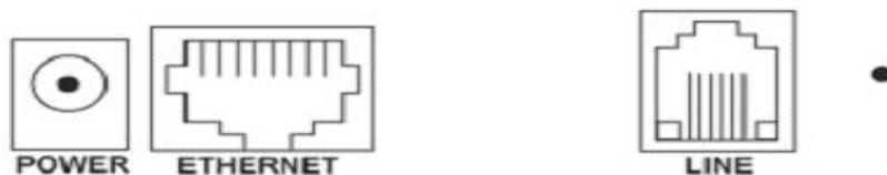
Figure 2) SiPTel IP Phone Rear Panel
