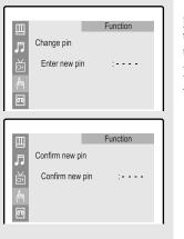
→ Note: If you forget the PIN, press the remote-control buttons in the following sequence, which resets the pin to 0-0-0: POWER OFF → MUTE → 8 → 2 →
