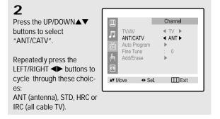
Note: STD, HRC and IRC identify various types of cable TV systems. Contact your local cable company to identify the type of cable system that exists in your particular area.
