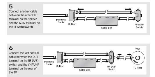
After you've made this connection, set the A/B switch to the "A" position for normal viewing. Set the A/B switch to the "B" position to view scrambled channels. (When you set the A/B switch to "B," you will need to tune your TV to the cable box's output channel, which is usually channel 3 or 4.)
