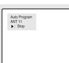
✓ The TV automatically cycles through all of the available channels and stores them in memory. This takes about one to two minutes. Press the RIGHT ▶ button at any time to interrupt the memorization process and return to the Channel menu.
