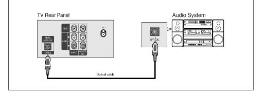
Connect an optical cable between the DIGITAL AUDIO IN jacks on the AUDIO and the DIGITAL AUDIO OUT jack on the TV.
