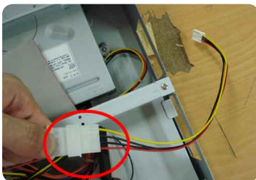
Connect to the power cable
