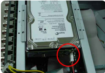
Connect to the power cable
