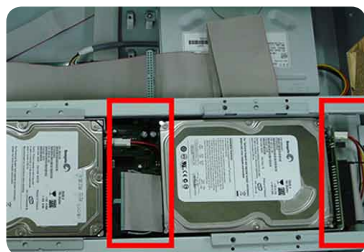
Connect to the E-IDE HDD cable
