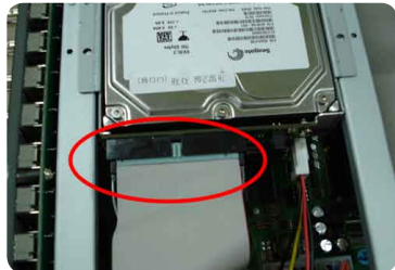
Connect to the E-IDE HDD cable
