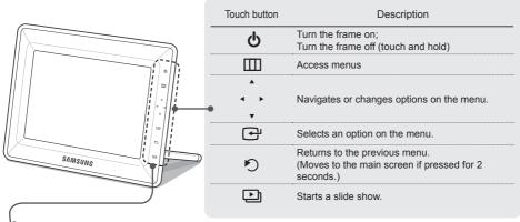
**Caution:** While the photo frame is booting, do not press and hold the touch buttons. Touch buttons pressed while the photo frame is booting will not operate.
