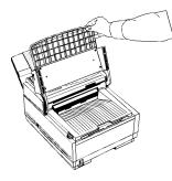
2 Push in the cover release buttons on the side of the copy stacker until you hear a click. Lift the copy stacker.
