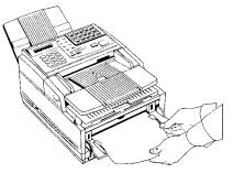
6 Press the Copy key (refer to the instructions above). If you are making more than one copy, or copying a multi-page document, insert additional sheets when the previous sheet is all the way through the machine.
