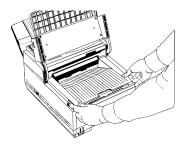
**3** Pull the blue lever on the old toner cartridge all the way toward you. Carefully pull the old toner cartridge out of the image drum unit. Dispose of it in the plastic bag you received with your new cartridge.
