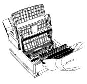
**4** Remove the protective sheet. Be careful not to touch the green surface of the drum.
