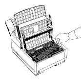
4 Push the lever forward to secure the cartridge.
