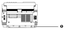
**6** Insert the end of the cord into the TEL 1 or TEL 2 jack on the back of the fax machine.
