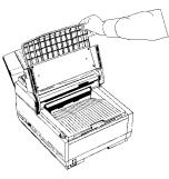
**2** Push the buttons on the side of the copy stacker until you hear a click. Lift the copy stacker up.
