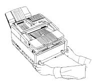
**3** Pull the manual paper feeder down until it is horizontal.
