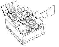
2 Neatly stack your documents, then insert them face down into the document feeder. Readjust the document guides for a snug fit. Your fax machine will grip the documents, and pull the bottom page into the machine.
