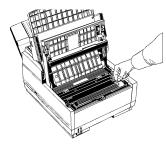
7 Using the cleaning wipe provided with your new toner cartridge, gently wipe back and forth across the full length of the LED array. Let the array dry completely.
