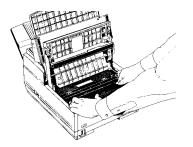
6 Install a new toner cartridge. Remove the new toner cartridge from its package and gently shake it from side to side to distribute the toner. Then carefully peel the white plastic tape from the bottom of the toner cartridge.
