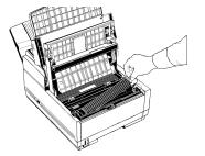
6 Once the toner cartridge is in place, push the lever all the way toward the back of the fax machine to secure it and release the toner.
