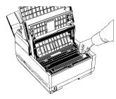
**9** Using the cleaning wipe provided with your new toner cartridge, gently wipe back and forth across the full length of the LED array. Let the array dry completely.
