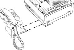
**3** Plug one end of the handset cord into the handset and the other end into the jack on the front of the cradle. Place the handset in the cradle.
