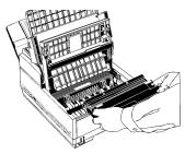
4 Remove the protective sheet from the new image drum unit.
