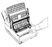
**5** Pull out the paper tray. If any paper in the tray is damaged, remove and replace it.
