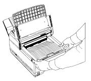
3 Lift the image drum cartridge out and set it aside.
