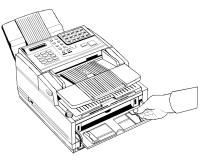
**5** Insert a sheet of paper face up. Adjust the guides again to ensure that the paper is straight.
