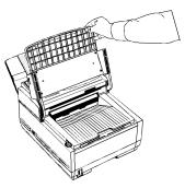
2 Push in the cover release buttons on the side of the copy stacker until you hear a click. Lift the copy stacker.
