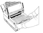
**3** Remove the old image drum unit (with its toner cartridge), wrap it in the packaging materials from your new image drum unit, and discard it.
