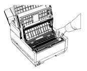
4 Remove the new toner cartridge from its package and gently shake it from side to side to distribute the toner. Then carefully peel the white plastic tape from the bottom of the toner cartridge.
