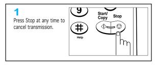
The fax transmission is canceled and the machine returns to Standby Mode.
