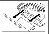
Wipe the roller and the thermal head with a soft cloth dampened with water.
