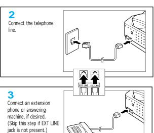
Plug one end of the telephone line cord into the TEL LINE jack and the other end into a standard telephone wall jack.
