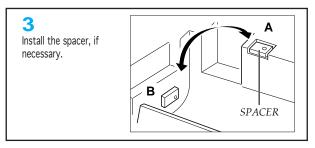
✓ If your paper roll is 8.5 in/216mm wide (letter size), the spacer should be in position "A". For narrow paper (A4 size, 8.27 in/210mm), place the spacer in position "B", pushing its pins into two small holes on the left-hand wall of the paper compartment.
