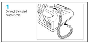
Plug the coiled cord into the HANDSET jack on the left side of the machine.
