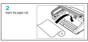
◄ If there is an adhesive sticker sealing the paper roll, remove it completely.
