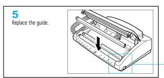
Make sure the handles on the end of the roller lock in place.
