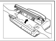
Cut off any wrinkled paper from the end of the paper, making the end straight and neat.
