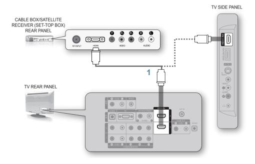
1. Connect an HDMI Cable (Not supplied) between the HDMI IN (1, 2 or 3) jack on the TV and the HDMI jack on the Cable Box/Satellite receiver (Set-Top Box).
