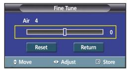
Press the ◀ or ▶ button to adjust the fine tuning.
