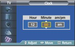
Press the ▶ button to select "am/pm", then press the ▲ or ▼ button to select the proper time of day (am or pm).
