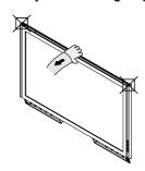
Hold onto the middle of the PDP to adjust the angle (not the sides of the PDP).
