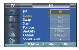
Press the ▲ or ▼ button to cycle through all of the available signal sources: "TV", "AV1", "AV2", "AV3", "S-Video1", "S-Video2", "Component1", "Component2", "PC", and "DVI".
