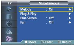
Press the ▲ or ▼ button to select "Fan", then Press the ENTER button.
