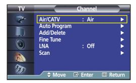
Press the  $\blacktriangle$  or  $\blacktriangledown$  button to select "LNA", then press the ENTER button.
