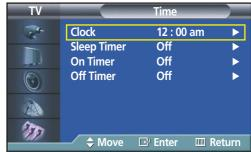
Press the ENTER button to select "Clock", then press the ▲ or ▼ button to select correct hour.
