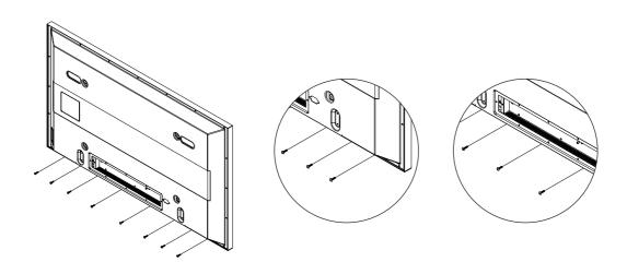
Set the Speaker Guide Bracket into the square grooves located on either side of the PDP's bottom rear, then push the Speaker Guide Bracket towards the center (as the arrow illustrates). Secure the Speaker Guide Bracket with provided screws. Secure the Middle Cabinet to the center of the PDP with a screw. (Always use the proper screws, as indicated.)
