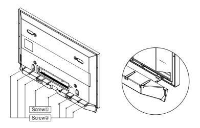
Secure the Speaker Dust Cover by setting it into the grooves located on the front side of the speakers.
