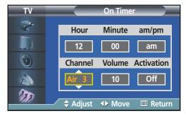
Press the ▶ button to select "Volume", then press the ▲ or ▼ button to select the volume level you want when PDP turns on.
