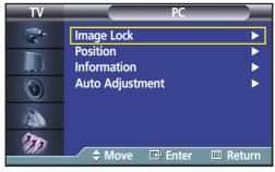
Press the ▲ or ▼ button to select "Information", then press the ENTER button. The vertical, horizontal frequencies and resolution appear.
