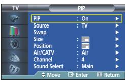
Press the ▲ or ▼ button to select "Position", then press the ENTER button.
