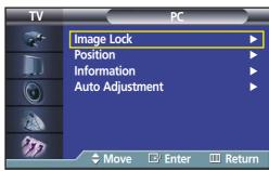
Press the ▲ or ▼ button to select "Auto Adjustment", then press the ENTER button. The message "Auto Adjustment in progress." appears on the screen and the picture adjustments are automatically activated.
