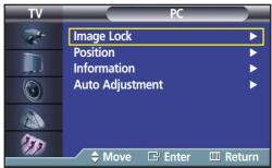
Press the ▲ or ▼ button to select "Position", then press the ENTER button.
