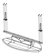
2 Using the 4 screws for securing the Stand Pegs and the Monitor, firmly attach the Monitor to the Stand Pegs. (The exterior of the SET may be different than the picture.)
