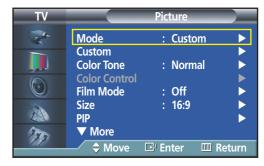
Press the ▲ or ▼ button to select "Film Mode", then press the ENTER button.
