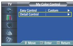
Press the ▲ or ▼ button to select "Detail Control", then press the ENTER button.
