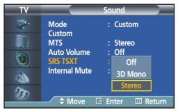
Press the ▲ or ▼ button to change the setting (Off, 3D Mono or Stereo), then press the ENTER button.
