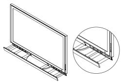
Connect the speakers to the PDP using the speaker cable.
