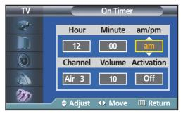
Press the ▶ button to select "Channel", then press the ▲ or ▼ button to select the channel you want when PDP turns on.
