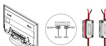
When you connect the speaker wire to the external speaker out connector, first bind the speaker wire round the ferrite core to secure it.
