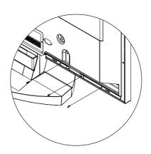
2 Set the Speaker Guide Bracket into the square grooves located on either side of the PDP's bottom rear, then push the Speaker Guide Bracket towards the center (as the arrow illustrates). Secure the Speaker Guide Bracket with provided screws. (Always use the proper screws, as indicated.)
