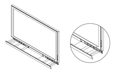
Connect the speakers to the PDP using the speaker cables.
