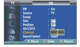
Press the ▲ or ▼ button to change the channel that appears in the PIP window.
