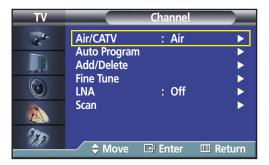
Press the ▲ or ▼ button to select "Fine Tune", then press the ENTER button.
