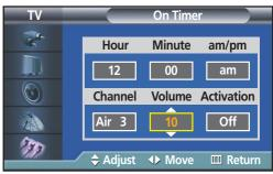
Press the ▶ button to select "Activation", then press the ▲ or ▼ button to select "On" or "Off".
