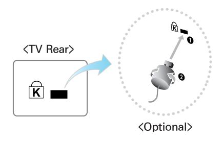
A Kensington Lock is a device you can use to physically fix your TV in place when using it in a public place.
