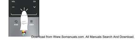
Press the  $\bullet \bullet \bullet$  button in the bottom center of the Touch Pad. You can select a desired function (e.g. Menu( $\blacksquare$ ), Source( $\bullet$ ), Info(i), etc.) easily.
