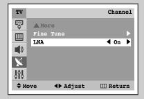
This function is very useful in the situation that the TV is used in weak signal. LNA amplifies the TV signal in the weak signal area, but not noise. This feature is working only weak signal condition, and that is memorized on current channel, additional.
