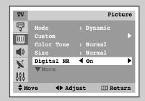
If the signal received by your television is weak, you can activate this feature to reduce any static and ghosting that may appear on the screen.
