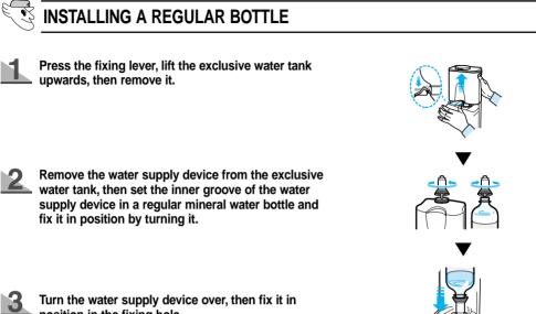
Turn the water supply device over, then fix it in position in the fixing hole.
