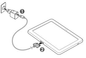
Connecting the USB cable improperly may cause serious damage to the device or USB power adapter. Any damage caused by misuse is not covered by the warranty.
