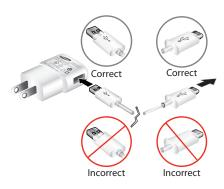
2. Insert the USB cable into the device's Charger/ Accessory Port.
