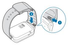
**Note:** If you replace the strap on your Gear 2<sup>™</sup> with another strap not manufactured by Samsung, please use a strap with a standard 22mm spring bar pin, and refer to the manufacturer's instructions to properly attach the band.
