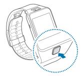
2. Press and hold the Power button, and then tap Power off to turn off the Gear 2™.
