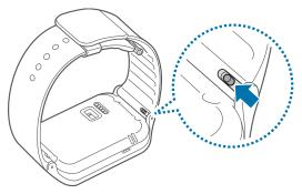
2. Lift the strap out to detach it from the Gear 2<sup>™</sup>.
