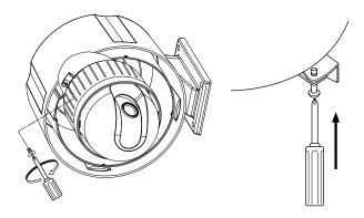
**9** For smooth assembly of the dome, apply silicon grease to the gasket, align it with the boss and push the dome vertically into the housing.
