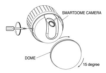
Align the arrow on the camera adaptor with the arrow on the Smartdome Camera, insert the three bosses on the back of the camera into the three camera adaptor holes, together with the connectors, and turn the camera about 15 degrees clockwise. (Listen for the click that confirms engagement and make sure that the locking lever returns to its original position.)
