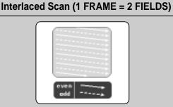
In interlaced-scan video, a frame consists of two interlaced fields (odd and even), where each field contains every other horizontal line in the frame. The odd field of alternating lines is displayed first, and then the even field is displayed to fill in the alternating gaps left by the odd field to form a single frame. two interfaced fields, thus a total of 60 fields are displayed every 1/60th of a second each.
