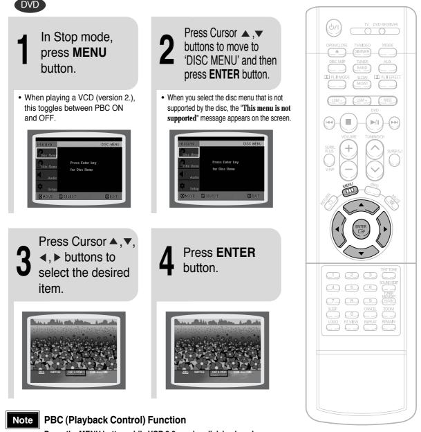
Press the MENU button while VCD 2.0 version disk is played. Each time you press the button, "PBC ON" and "PBC OFF" will be repetitively selected in the display.
