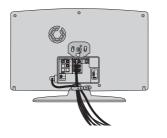
Use the cable tie to keep the cables together.
