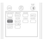
In Stop mode, press and hold the **SD/HD** (Standard Definition/High Definition) button on the remote control.
