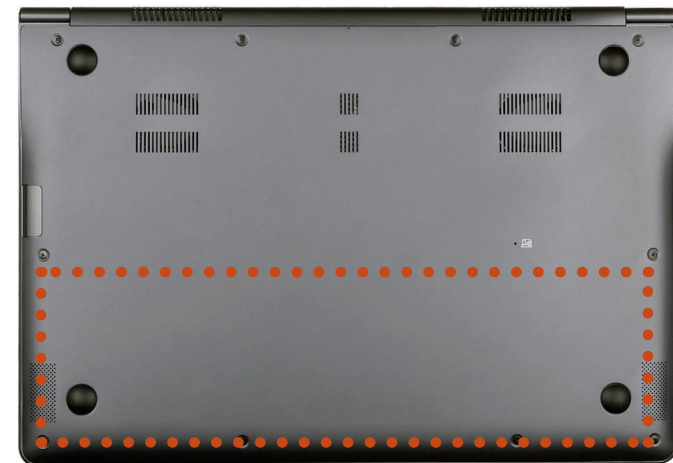
The location of the internal battery
