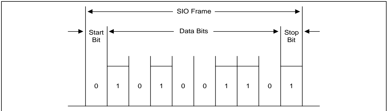
Figure 11-4. Serial I/O Frame Timing Diagram (Normal UART)
