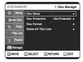
Press the ▲▼ buttons to select **Disc Name**, then press the **ENTER** or ▶ button.
