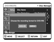
Press the ◀▶ buttons to select **Yes**, then press the **ENTER** button. The disc is formatted.
