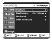
Press the ▲▼ buttons to select **Disc Protection**, then press the **ENTER** or ▶ button.
