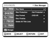
Press the ▲▼ button to select **Disc Finalize**, then press the **ENTER** or ▶.
