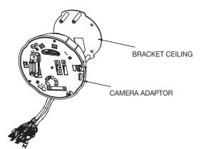
5. Remove the Connectors at the end of the Camera Adaptor.
