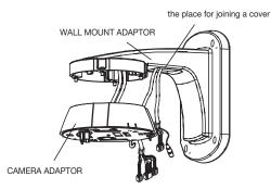
7. Insert the 4 screws on the Wall Mount Adaptor into the corresponding screw holes on the Camera Adaptor and fix them so that the Camera Adaptor is secured to the Wall Mount Adaptor.
