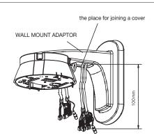
9. Use the anchor bolts and nuts to secure the Wall Mount Adaptor to the wall.
