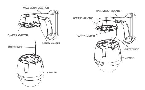
13. Align the Guide 1 of the Camera with the Guide 2 of the Camera Adaptor and insert the 3 Guides of the Camera into the corresponding Guide Holes of the Camera Adaptor. Then, turn the camera clockwise by 10 degrees.
