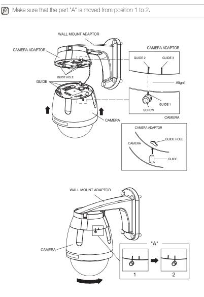
**14.** Use the screws, attached to the Camera, to firmly fix the Camera body with the Camera Adaptor.
