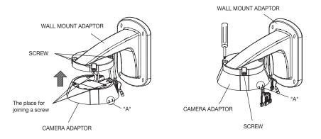
8. Pull out cables such as external power cable, BNC cable and communications cable through the rear of the Wall Mount Adaptor, which are necessary for connecting the camera.
