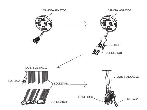
6. Prepare the Camera Adaptor for the applicable camera. Refer to the installation guide for the applicable camera and configure the initial settings of the Camera Adaptor. (For more information, see the installation guide for the Camera) Insert the cable of the Camera Adaptor into the Wall Mount Adaptor before pulling it out throught the hole of the Cover Fixing Part.
