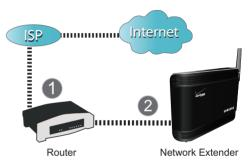
Connect one end of the included Ethernet cable to an open port on the router (1) and connect the other end to the WAN port located at the rear of the base station (2).
