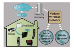
About the size of a traditional wireless access point (WAP), the base station facilitates the delivery of cellular traffic through the Internet to the Verizon Wireless network, which then routes the signal to the desired party.
