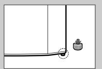
To compensate for an uneven floor surface, you can adjust the feet on the front of the fridge/freezer.
