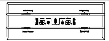
**Freezer Temp** : Indicates the current freezer temperature. **Fridge Temp** : Indicates the current fridge temperature.
