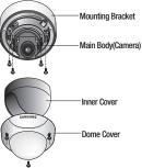
2. And then remove the main body from the mounting bracket by the four main body screws. Adjust the panning, tilting and rotate mechanism while checking the position on the monitor
