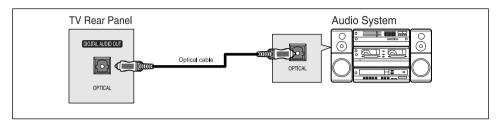
Connect an optical cable between the DIGITAL AUDIO IN jacks on the AUDIO and the DIGITAL AUDIO OUT jack on the TV.
