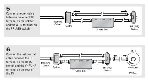
After you've made this connection, set the A/B switch to the "A" position for normal viewing. Set the A/B switch to the "B" position to view scrambled channels. (When you set the A/B switch to "B," you will need to tune your TV to the cable box's output channel, which is usually channel 3 or 4.)
