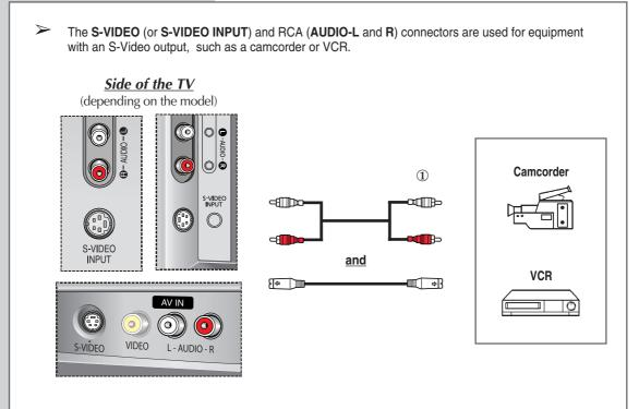
① To play pictures and sound, both the S-VIDEO (or S-VIDEO INPUT) and RCA connectors must be used.
