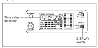
Use the DISPLAY switch to switch time value indications
