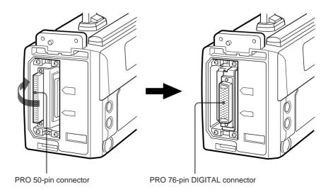
**3** Attach the cover upside down. Make sure that the match mark lines up with the PRO76P DIGITAL indication.
