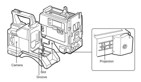
**3** Slide the DSR-1/1P along the groove on the camera, and press firmly until fixed.
