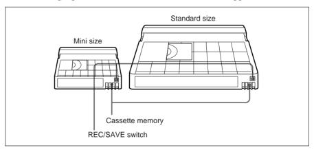
For ClipLink shooting, a DVCAM cassette including "cassette memory" is necessary. In the cassette memory, data required for editing the recorded video (ClipLink log data) is stored. The DSR-1/1P can record or play back the cassettes with cassette memory of 16 kbits or less.
