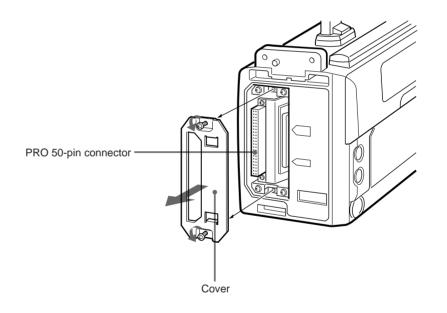
**2** Press the right side of the PRO 50-pin connector until the PRO 76-pin DIGITAL connector appears.
