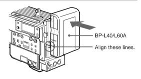
2 Slide the battery pack down until its "LOCK" arrow points at the matching line on the DSR-1/1P.
