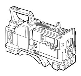
**4** Tighten the two screws (M4  $\times$ 12) in the figure.
