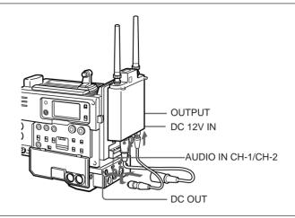
**4** Set the AUDIO IN (CH-1/CH-2) switch (for the tunerconnected channel) to REAR and the input selection switch for the AUDIO IN CH-1/CH-2 connector (where the tuner cable is connected) to MIC (center position).
