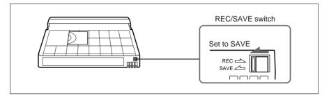
If you insert a cassette into the DSR-1/1P when this switch is set to SAVE, the DSR-1/1P will not record when you press the REC button.
