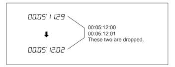
In non-drop-frame mode, however, no frame counts are omitted, and there is a gradual deviation of the time code from real time.
