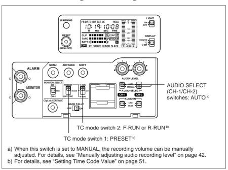
**4** Display menu 212 and select the audio recording mode (two-channel mode or four-channel mode).
