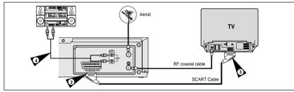
You can connect your VCR to the television using the SCART cable if the appropriate input is available on
