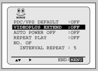
To prevent delays or over-runs the VCR has a function called Videoplus EXTEND allowing you to extend the recording time by up to 60 minutes.
