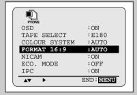
Your VCR can automatically play Wide Screen format prerecorded tapes. It can also record Wide Screen format programmes received from sources such as a satellite receiver.
