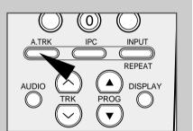
The Picture Alignment feature enables you to optimize the tape position automatically to obtain the best possible picture.
