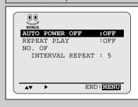
The Auto Power Off feature automatically turns off your VCR if no signal is received and you do not press any button for the selected time.
