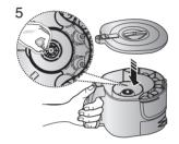
After empting the DUST BIN, remove the obstacles like hair, fur on the cap of the DUST BIN.
