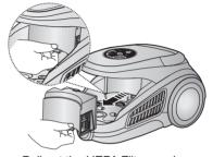
Pull out the HEPA Filter as shown.
