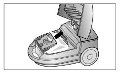
3) After removing the used dust bag, insert the cardboard bag collar of the new dust bag into the suction inlet to the full.
