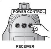
Press the power control button repeatedly to select the correct mode.
