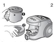
Remove the dust bin and dust pack as shown.
