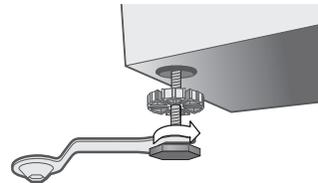
7. Level your Washer by turning the leveling legs in or out as necessary by hand or wrench included with your Washer. When your Washer is level, tighten the nuts using the wrench or (-) driver.
