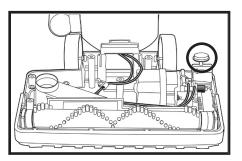
5 Make sure the reset button cover (circled) is in position on spring. Replace hood. Hold body and power nozzle, turn over so bottom of power nozzle is facing up. Replace screws.
