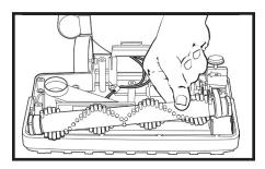
(3) Place the other end of belt around brush roll. Align left end of brush roll into the base by rotating slightly until brush roll end cap slides into place.
