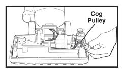
(2) Remove broken brush roll belt. Pinch new brush roll belt together and position new belt so teeth engage cog pulley on end of motor shaft.
