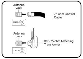
Connect the 75 ohm cable from the combination VHF/UHF antenna to the antenna jack.
