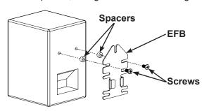
Slide the Speaker and EFB onto the L-Bracket on the stand.
