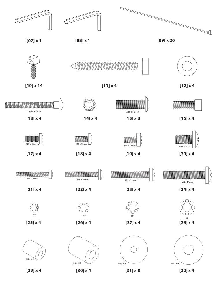
Determine the Bolt diameter required — [17] / [21], [18] / [22], [19] / [23], or [20] / [24] — by threading each size into the back of the TV. Stop immediately if you encounter any resistance.
