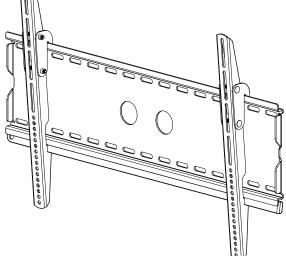
Thank you for choosing the Sanus Systems Vision Mount wall mount. The Sanus Systems VMPL2 wall mount is designed to support a monitor weighing up to 79 kg (175 lbs) to a vertical wall either flat or at a fixed 5 degree tilt. Hardware for multiple mounting configurations is included.
