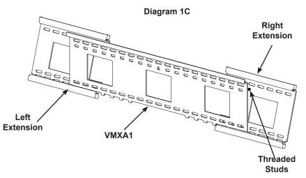
Using the previously removed Flange Nuts and Nylon Washers, secure the Right and Left Extension to the VMXA1 as shown in Diagram 1D, and securely tighten the Flange Nuts.
