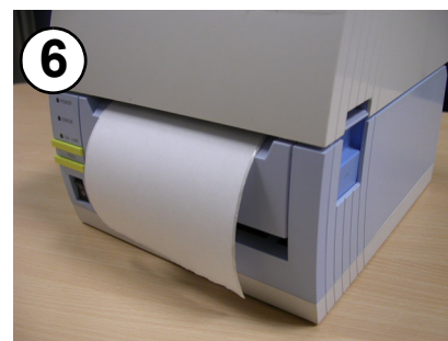
6 Close the cover. Direct thermal printing is now possible.
